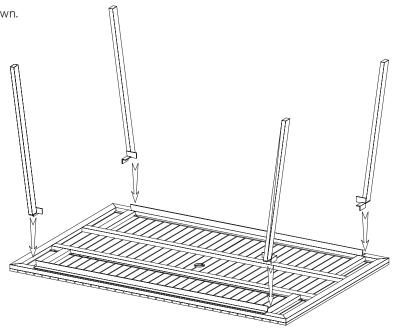
2. Fasten legs to frame using bolts (A) as shown. Put all 20 bolts in loosely before tightening with allen key (B).
