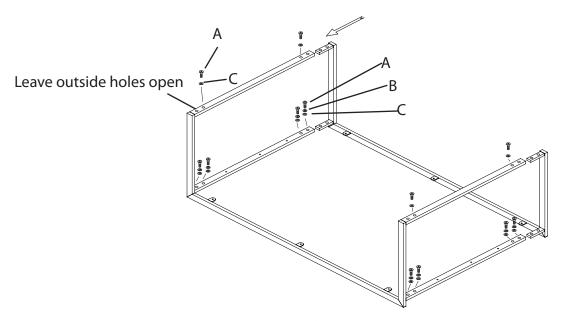
2. Insert adjustable levelers (D) into the holes left open in step 1. These levelers can be adjusted after the table is flipped over to conform to uneven flooring.
