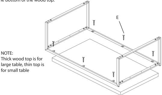
4. Attach the wood top using wood screw (F) thru the end rails into the bottom of the wood top. Once the wood top is attached tighten all bolts using the supplied allen key.
