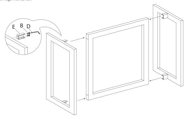
3. Connect legs to center using short bolts (B) as shown. Tighten bolts using allen key (D).
