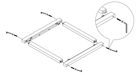
2. Fasten corner legs to frame using bolts (A) as shown. Tighten bolts using allen key.
