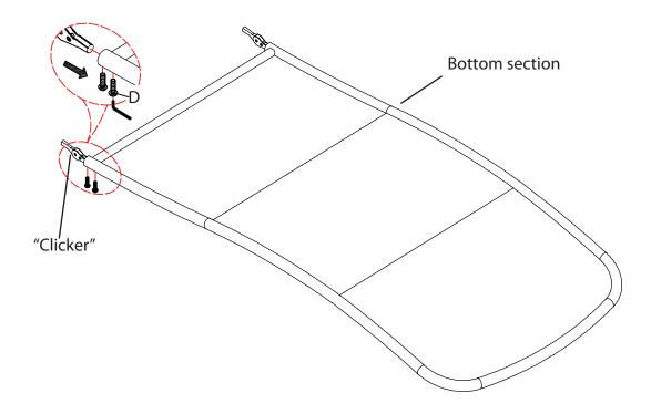
3. Align bottom section onto assembled frame like the drawing shows. insert bolt (A), lock washer (B) & flat washer (C) into the bottom of the rails through into the bottom section of the lounger.
