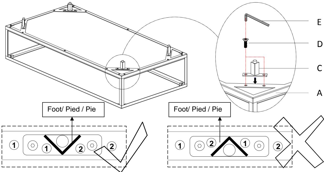
2. Carefully turn the table upright, lift the Glass (B) and gently put it onto the frame as shown. Adjustable levelers are installed to accommodate uneven flooring. To adjust these levers, simply turn them clockwise to up or counterclockwise to down.
