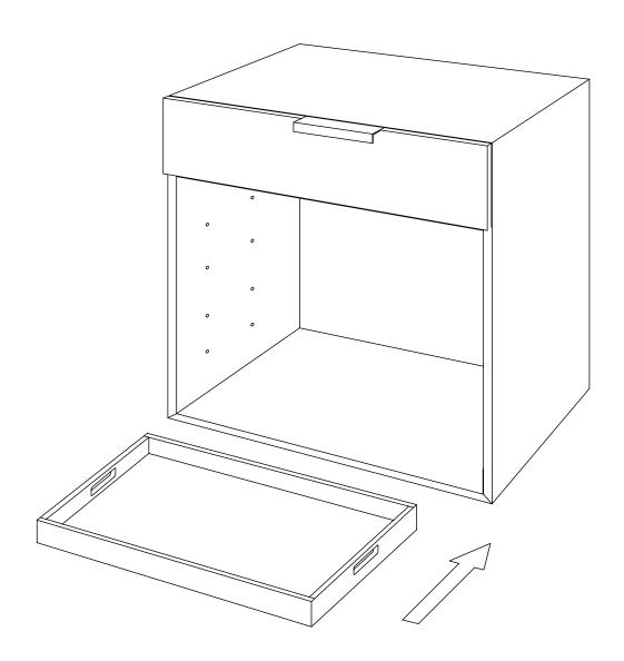
9375817 - 05/07 Page 3 of 6 3. Insert shelf pins (A) into cabinet holes as shown. Set shelves on pins.
