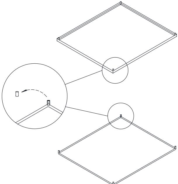
2. Align posts (C) with the bottom frame as shown. Insert set screws (D). Tighten with supplied hex key (E). Repeat for top frame.
