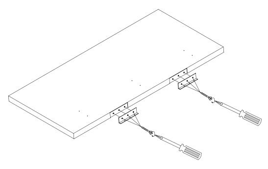
2. Align the holes in the triangle blocks with the holes on the headboard. Attached the triangle blocks to the headboard and secure them with 2 screws (B) for each block.
