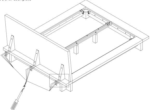
5. Make sure to install all screws as shown in the drawing. 2 screws in the block and 2 screws in the bedframe per rectangular bracket (D).
