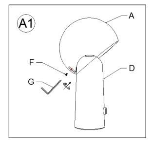
Attach the Shade (A) onto the bracket of Base (D), making sure the screw holes on both parts are aligned. Insert the Screw (F) and fasten with an Allen Key (G). Rotate screw clockwise until tight.
