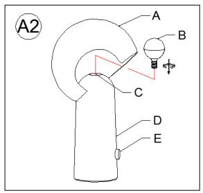
Insert the specified light bulb into the Socket (C).DO NOT EXCEED THE SPECIFIED WATTAGE.
