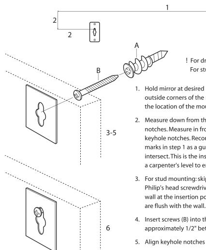
! For drywall mounting, use anchors with screws. For stud mounting, use screws only.
