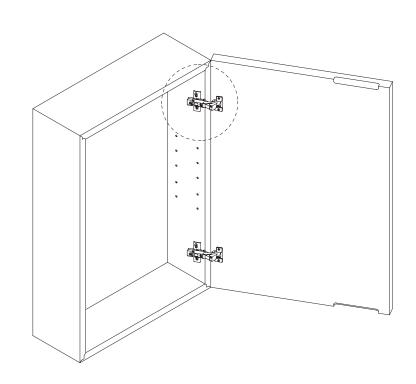
2. Screw in shelf pins (A) at desired locations inside cabinet. Set glass shelves onto shelf pins.
