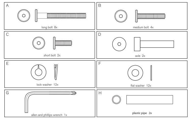
1. Fasten back legs to desk top using flat washer (F), lock washer (E), and long bolt (A) in order as shown. Tighten with allen wrench (G).
