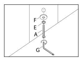
2. Fasten front legs to desk top using flat washer (F), lock washer (E), and medium bolt (B) in order as shown. Tighten with allen wrench (G).
