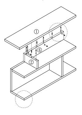
6. if your bookshelf side table does not sit level on your floor you will need to adjust the levlers on each corner to accomodate uneven surfaces. Clockwise tightens raises the leveler and counterclockwise lowers the leveler. You may need to adjust more than one leveler to get the shelves level.
