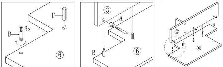
3. insert dowel (F) into bottom of part #3. Screw cam bolt (B) into the bottom of part #3. Insert cam lock (A) into the side of part #4. Press part #4 onto part #3 as the drawing shows. Turn cam lock 1/2 turn with phillips head screwdriver to tighten.
