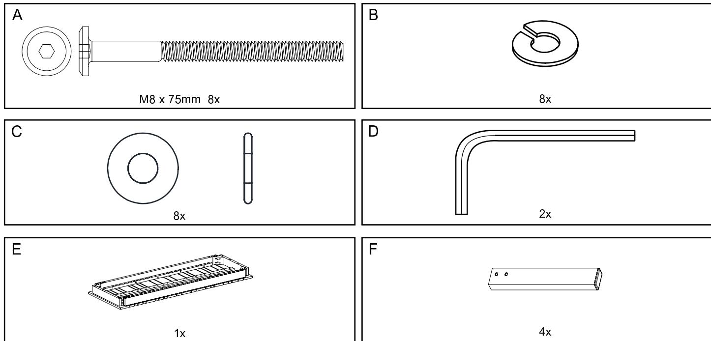
1. Lay the bench seat (E) upside down onto a clean smooth surface such as carpet or cardboard. Align legs (F) as shown. Insert bolt (A), lock washer (B), and flat washer (C). Tighten with supplied hex key (D). Stand bench upright and sit on it for 5 minutes, then retighten all bolts.
