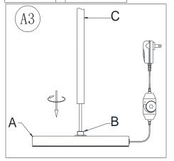
3. Gently pull and remove any slack power cord out from the Base (A). Attach the Lower Tube (C) onto Thread Nipple (B) of Base (A) by rotating the Lower Tube (C) in a clockwise direction until tight.
