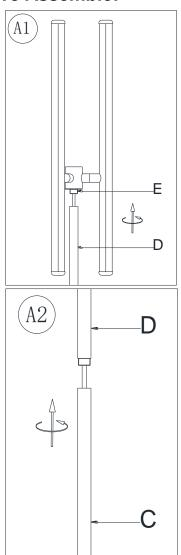
1. Attach the Upper Tube (D) onto the bottom threaded end of Light Rods Assembly (E) by rotating the Upper Tube (D) in a clockwise direction until tight.
