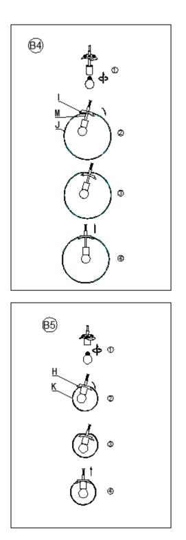
4. Insert the specified light bulb into the socket. DO NOT EXCEED THE SPECIFIED WATTAGE. Insert the stem(M) into the large glass(J) in a slant angle. And make sure the stem(M) to hold large glass (J) in place.
