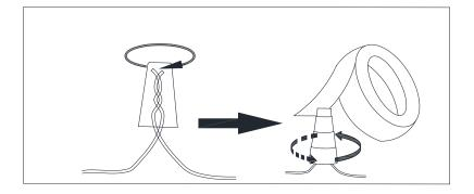
Connect the GROUND FIXTURE WIRE to the GROUND J-BOX WIRE using the Plastic Wire Nut Connector (N) and wrap the connection with electrical tape. Be sure that no wire strands are exposed.
