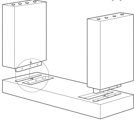
2. Attach the flat washer (B) and lock washer (C) with bolt (A). Tighten with allen key (D).
