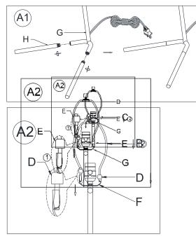
Attach the Bottom Tube (H) into Joints (G) by turning each Bottom Tube (H) clockwise until tight.
