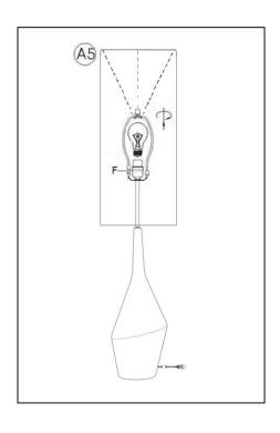
Insert the specified light bulb into the Socket (F). DO NOT EXCEED THE SPECIFIED WATTAGE.
