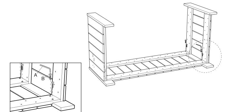
2. Fasten bench sides to to front as shown. Tighten bolts (B) using allen key (A).
