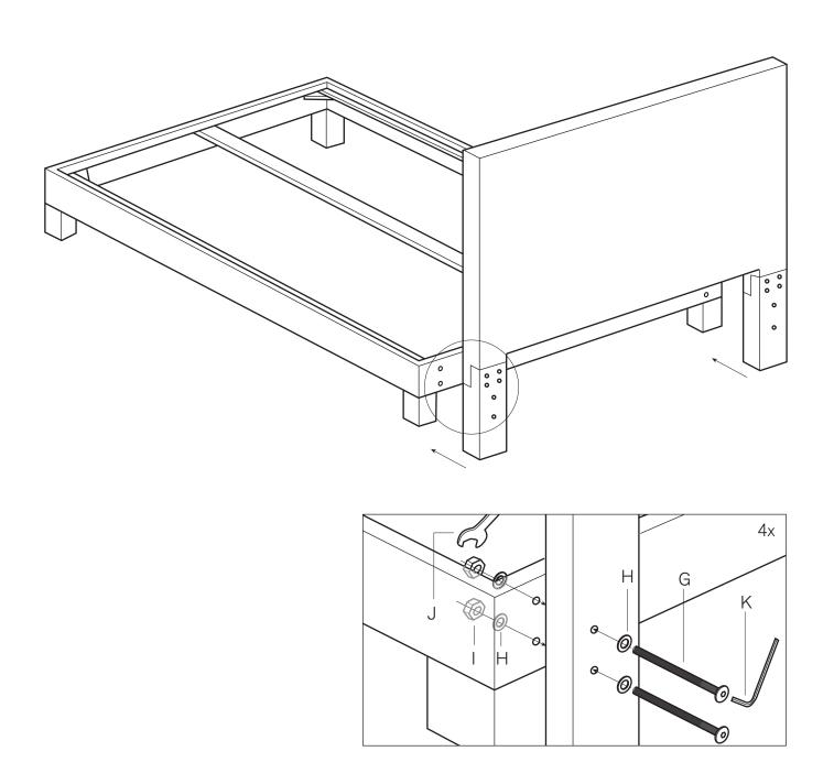
Attaching the headboard to tall wood bed frame:
