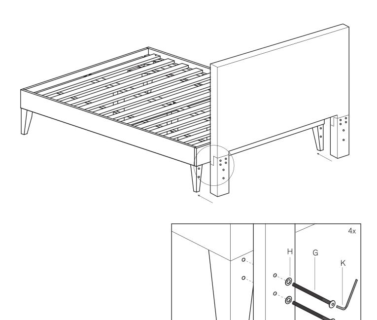
Attaching the headboard to standard metal frame:
