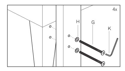
Attaching the headboard to narrow leg bed frame
