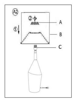
Place the Shade (B) over onto the Socket (C) and secure the shade in place by turning the Socket Ring (A) in a clockwise direction until tight.
