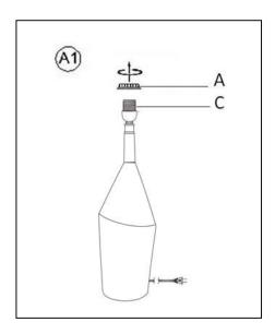
Unscrew Socket Ring (A) from Socket (C) by turning counter-clockwise.
