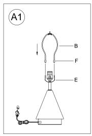
1. Raise the Harp Caps (F) and insert the bottom ends of Harp (B) into the Saddle (E)
