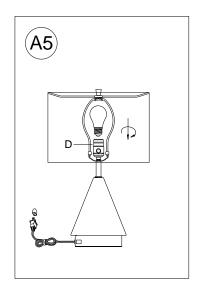
Insert the specified light bulb into the Socket (D). DO NOT EXCEED THE SPECIFIED WATTAGE.
