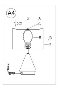
4. Place the Shade (G) over the Harp (B) making sure the Harp Top (C) extends through the top ring of Shade (G). Secure the Shade (G) by turning the Finial (A) onto the Harp Top (C).
