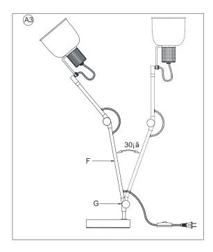
3. If needed, loosen the Lower Clamping Nut (G) and adjust the Lower Tube (F) to your desired angle, then retighten the Lower Clamping Nut (G) clockwise until secure. Do not exceed the adjustable angle as the diagram illustrated.
