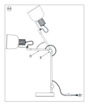
4. If needed, loosen the Upper Clamping Nut (E) and adjust the Upper Tube (D) to your desired angle, then retighten the Upper Clamping Nut (E) clockwise until secure.
