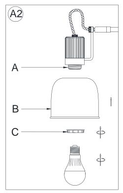
Attach the Shade (B) onto the Socket (A). Secure Shade
