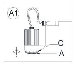
1. Unscrew the Socket Ring (C) from the Socket (A) by rotating counter-clockwise.
