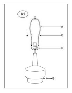
Raise the Harp Caps (E) and insert the bottom ends of Harp (D) into the Saddle (G)  $% \left( G\right) =0$
