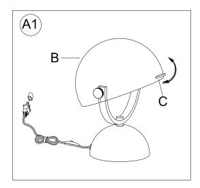
1. If needed, adjust the Metal Shade (B) to the desired angle by gently moving the shade handle (C) until it is determined.
