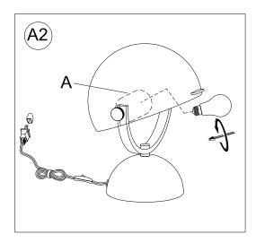
Insert the specified light bulb into the Socket (A). DO NOT EXCEED THE SPECIFIED WATTAGE.
