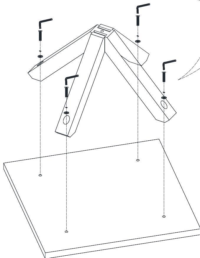
2. Align bottom leg frame with assembly from step 1. Make sure to align tenons into slots in frames. Insert bolt (B), lock washer (C), flat washer (D), and tighten with supplied hex key (E). With help carefully flip the table up right without leaning it on the legs as you turn it over. This could cause damage to the table.
