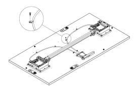
**Step 5:** Use handle assembly to release the mechanisms and lock in the upright position.
