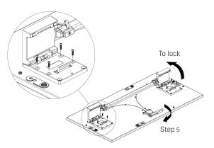
**Step 7:** Use handle assembly to release the mechanisms and return to lowered position. Attach each leg with enclosed M6 Truss Phil screws.
