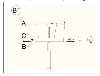
Separate the Mounting Plate (A) from the Canopy (C) by removing the 3 Canopy Screws
