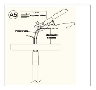
5. If needed, cut off the extra power cord length on the 2 cord wires and bare ground wire, so that they are at least 6 inches (152.4 mm) long within the outlet junction box (J-box).
