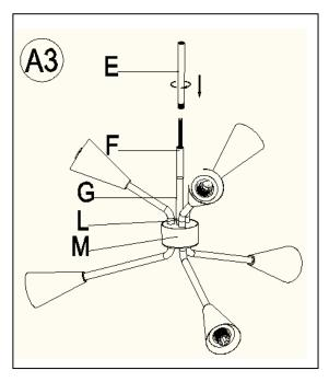
3. If you would like to use only 12 inch Tube (E), then thread the 3 wire power cords through the 12 Inch Tube (E), making sure the tube nipple joint end is downward as shown in diagram A3. Attach the bottom end of 12 Inch Lamp Tube (E) onto the top end of 6 in. Tube (F) and rotate clockwise until tight. If more 12 inch Tubes (E) are required, just follow above step.
