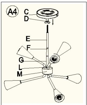
4. Once the fixture's suspension length is determined, thread the 3 wire power cords through Ball Joint (D) and Canopy (C). Attached the Ball Joint (D) onto the 6 inch Tube (F) or 12 Inch Tube (E) and rotate clockwise until tight.
