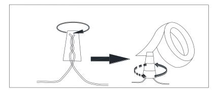
Connect the GROUND FIXTURE WIRE to the GROUND J-BOX WIRE using the Plastic Wire Nut Connector (Q) and wrap the connection with electrical tape. Be sure that no wire strands are exposed.
