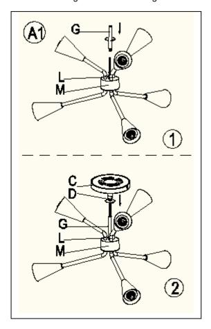
Insert the fixture 3 wire power cords through the 9.7 inch Tube (G), and attach bottom end of the 9.7 Inch Lamp Tube (G) onto the top end of Thread tube (L) and turning in a clockwise direction until tight.
