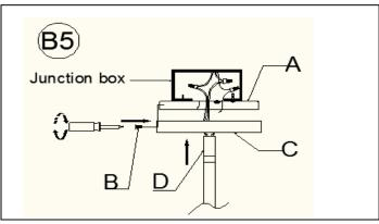
5. With the help of another people to hold the weight of the light fixture, Raise the Canopy (C) up over the Mounting Plate (A). Align the holes on the Mounting Plate (A) with the holes on the side of the Canopy (C). Insert the 3 Canopy Screws (B) and tighten with a screwdriver.
