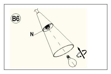
Insert the specified light bulbs into the Sockets (N).DO NOT EXCEED THE SPECIFIED WATTAGE.
