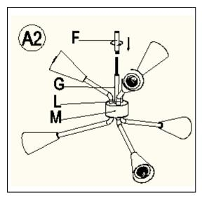
2. If you would like to use only 6 inch Tube (F), then thread the 3 wire power cords through the 6 Inch Tube (F), making sure the tube nipple joint end is downward as shown in diagram A2. Attach the bottom end of 6 Inch Tube (F) onto the top end of 9.7 inch Tube (G) and rotate clockwise until tight.
