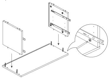
5. Slide back panel into groove. Make sure panel slides all the way into the bottom panel groove.
