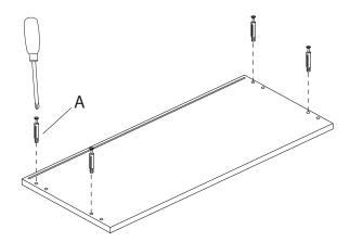
4. Fasten side panels to bottom panel. The bottom panel is indicated with a "Made in Denmark" sticker. Fit cam screws into cam locks and tighten using a phillips screwdriver.
