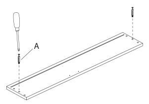
9. Fasten drawer side panels to drawer front panels. Insert small cam locks (C) into side panels. Fit cam screws into cam locks and tighten using phillips screwdriver.
