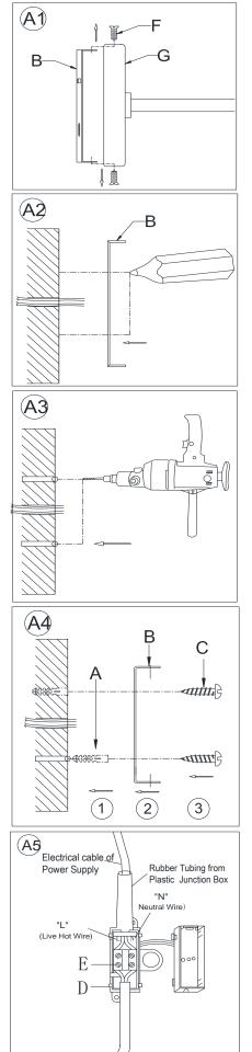
Separate the Mounting Plate (B) from the Canopy (G) by removing the 2 Canopy Screws (F). Do not discard the Canopy Screws (F) as these will be used later.
