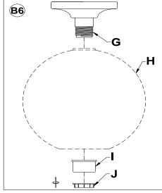
Put the Glass Shade (H) and Spacer (I) onto the Socket (G), secure Glass Shade (H) and Spacer (I) by rotating the Socket Ring (J) in a clockwise direction until tight. Do not over tighten.
