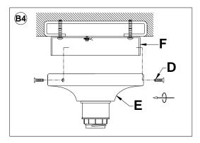
4. Position the Canopy (E) over the Mounting Plate (F), aligning the 3 holes on the Canopy (E) with the 3 holes on the Mounting Plate (F). Secure the Canopy (E) by tightening 3 Canopy Screws (D)
