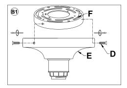
Separate the Mounting Plate (F) from the Canopy (E) by removing the Canopy Screws (D). Do not discard the Canopy Screws (D) as these will be used later.
