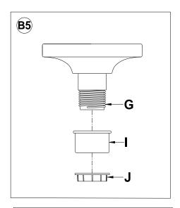
5. Unscrew the Socket Ring (J) and Spacer (I) from the Socket (G).
