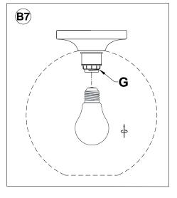
7. Insert the specified light bulb into the Socket (G). DO NOT EXCEED THE SPECIFIED WATTAGE.
