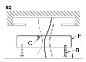
Insert the J-box wires through the center opening of Mounting Plate(F), Attach the Mounting Plate (F) onto the Wall J-box. Secure the Mounting Plate(F) by turning the 2 Mounting Screws(B) clockwise until tight
