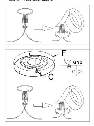
Connect the GROUND FIXTURE WIRE to the GROUND J-BOX WIRE using the Plastic Wire Nut Connector (A) and wrap the connection with electrical tape. Be sure that no wire strands are exposed.
