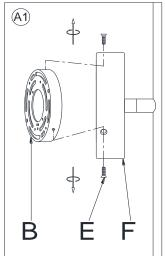
Separate the Mounting Plate (B) from the Canopy (F) by removing the Canopy Screws (E). Do not discard the Canopy Screws (E) as these will be used later.
