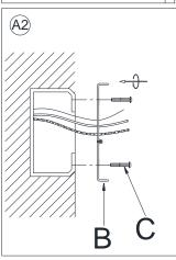
2. Insert the J-box wires through the center opening of Mounting Plate (B). Attach the Mounting Plate (B) onto the wall J-box. Secure the Mounting Plate (B) by turning the 2 Mounting Screws (C) clockwise until tight.
