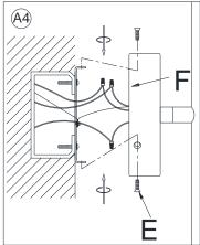
4. Position the Canopy (F) over the Mounting Plate (B), aligning the 3 holes on the Canopy (F) with the 3 holes on the Mounting Plate (B). Secure the Canopy (F) in place by tightening 3 Canopy Screws (E).
