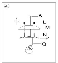
11. Unscrew the Knurled Nuts (L) from the Threaded Rods (N). Slide the Metal Cap (M) upwards along the Metal Tubes (J/K) and holding it with the help of another people.
