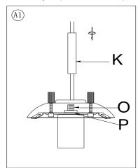
Attach bottom end of the Short Tube (K) onto the Threaded Pipe (O) by turning clockwise until tight.
