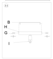
Separate the Mounting Plate (B) from the Canopy (H) by removing the 2 Canopy Screws (G). Do not discard the Canopy Screws (G) as these will be used later.
