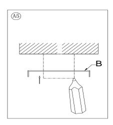
Determine your desired hanging location. Place the Mounting Plate (B) against the ceiling and mark the location of the slots of the Mounting Plate (B) onto the ceiling using a pencil.
