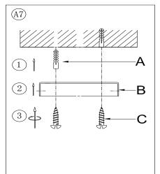
7. Insert each Plastic Anchor (A) into each drilled hole on ceiling. Attach the Mounting Plate (B) onto the ceiling aligning the 2 slots on Mounting Plate (B) with the 2 installed Plastic Anchors (A). Insert the Mounting Screws (C) and tighten each to secure the Mounting Plate (B) firmly onto the ceiling
