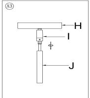
3. Attach the Swivel (I) onto the assembled Metal Tubes (J/K) by rotating the 2 parts clockwise until tight.
