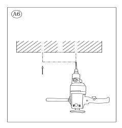
6. Using the drill with the appropriate size drill bit (just large enough to make hole that will allow passage of the Plastic Anchors (A) assemblies), drill one hole in the ceiling at each marked slot location for the Plastic Anchors (A).
