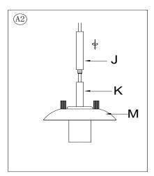
2. Attach the Long Tubes (J) onto the top of Short Tube (K) and rotate Long Tubes (J) clockwise until tight.
