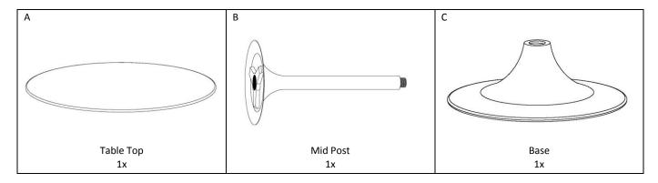
1. Tighten the mid post (B) to the Base (C) in the CW direction as shown below. Make sure that the mid post tightened fully with base.
