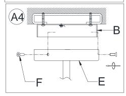
4. With the help of another person to hold the weight of lighting fixture, raise Canopy (E) up over the Mounting Plate (B). Align the 3 holes on the Mounting Plate (B) with the 3 holes on the side of the Canopy (E). Insert 3 Canopy Screws (F) and tighten to secure the Canopy (E) with a screwdriver.
