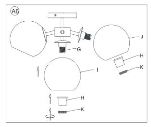
6. Attach the Large Glass Shade (I) onto the bottom Socket (G) and attach the four Small Glass Shades (J) onto the four side Sockets (G). Place the Spacers (H) onto the Sockets (G). Secure Glass Shades (I/J) and Spacers (H) by rotating the Socket Rings (K) in a clockwise direction until tight.
