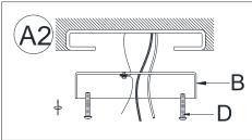
2. Gently pull existing wire down from the ceiling junction box and insert wires through the center opening of Mounting Plate (B). Attach Mounting Plate (B) to the ceiling outlet box, aligning the slots of the Mounting Plate (B) with the two threaded holes located on the J-Box. Insert and tighten 2 Mounting Screws (D) with a screwdriver.
