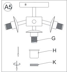
Unscrew the Socket Rings (K) and Spacers (H) from the Sockets (G) by rotating the Socket Rings (K) in a counter-clockwise direction.
