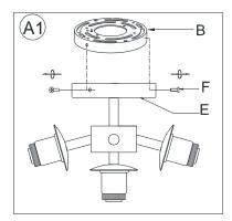
Separate the Mounting Plate (B) from the Canopy (E) by removing the 3 Canopy Screws (F). Do not discard the Canopy Screws (F) as these will be used later.
