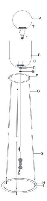
First attach 3 Tubes (G) into the 3 threaded nipples of Upper Ring (F) by rotating each Tube (G) in a clockwise direction until tight. Then attach the rest 3 Tubes (G) into the lower ends of assembled tubes.
