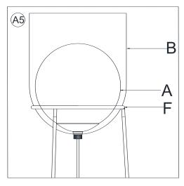
Gently place the assembled Glass Shades (A&B) onto the Upper Ring (F).
