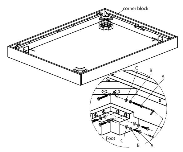
5. Align the holes in the top of the feet with the holes in the center rail. Insert bolts 8mm x 30 mm (F) and tighten with supplied allen key (G).
