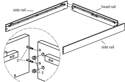
1. Screw in cam bolts (D) into holes in side rails as shown in drawing. Insert cam locks (E) into head rail as shown.
