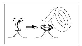
Connect the NEUTRAL FIXTURE WIRE to the NEUTRAL J-BOX WIRE first and then connect the HOT FIXTURE WIRE to the HOT J-BOX WIRE using the Plastic Wire Nut Connectors (A). Wrap these connections with electrical tape. Be sure that no wire strands are exposed.
