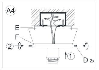
4. Raise Canopy (F) up over the Mounting Plate (E), align the holes in the Mounting Plate (E) with the holes on the side of the Canopy (F). Insert the 2 Canopy Screws (D) and tighten with a screwdriver.
