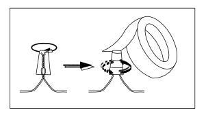
Connect the GROUND FIXTURE WIRE to the GROUND J-BOX WIRE using the Plastic Wire Nut Connector (A) and wrap the connection with electrical tape. Be sure that no wire strands are exposed.
