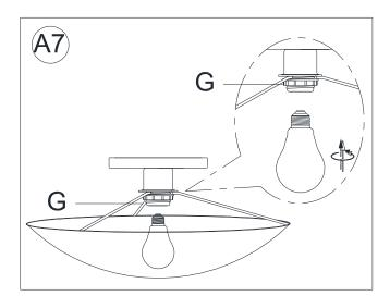
7. Insert the light bulb into the Socket (G). To avoid the risk of fire, do not exceed the recommended lamp wattage as outlined in Page 1.
