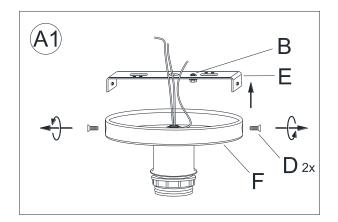
Separate the Mounting Plate (E) from the Canopy (F) by removing the 2 Canopy Screws (D). Do not discard the Canopy Screws (D) as these will be used later.
