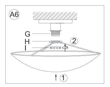
Raise Capiz Shade (H) (pack separately) over to the Socket (G). Turning Socket Ring (I) onto the Socket (G) till tight.
