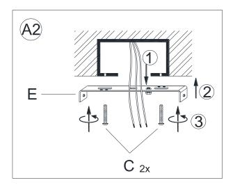
Gently pull existing wire down from the ceiling junction box and allow wires to hang. Attach Mounting Plate (E) to the ceiling outlet box. Tighten 2 Mounting Screws (C) with a screwdriver.
