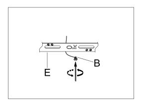
If the junction box DOES NOT has a GROUND WIRE, wrap the fixture's bare ground wire around the Green Ground Screw (B) and insert the screw into the Mounting Plate (E), marked as "GND", and tighten screw to secure the wire.
