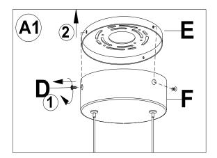
Separate the Mounting Plate (E) from Canopy (F) by removing the Canopy Screws (D). Do not discard Canopy Screws (D) as these will be used later.
