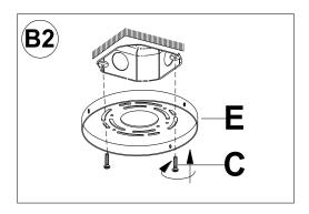
Gently pull existing wire down from the ceiling junction box and insert the wires through the center opening of the Mounting Plate (E). Attach the Mounting Plate (E) to the outlet box using the two J-Box Mounting Screws (C). Tighten each screw clockwise until the Mounting Plate (E) is firmly secured to the J-Box.
