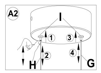
Press and hold the Cable Glider (I) upwards under the Canopy (F) and push the Power Cord (H) into the Canopy (F). Release the Cable Glider (I) once the desired fixture suspension length is determined. Adjust the Steel Cable(G) in the same way to make the light fixture level from left to right.
