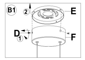
Separate the Mounting Plate (E) from Canopy (F) by removing the Canopy Screw (D). Do not discard Canopy Screws (D) as these will be used later.
