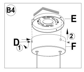
4. With the help of another person to hold the weight of the light fixture, position the Canopy (F) over the Mounting Plate (E), aligning the 3 holes on the Canopy (F) with the 3 holes from the Mounting Plate (E). Insert the 3 Canopy Screws (D) and tighten to secure the Canopy (F) in place.
