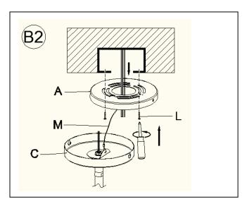
Insert the J-box wires through the center opening of the Mounting Plate (A). Attach the Mounting Plate (A) to the junction box using the two J-Box Mounting Screws (L). Tighten each screw clockwise until the Mounting Plate (A) is firmly secured to the J-Box. Then the steel wire (M) can hang up the fixture securely.
