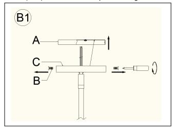
Separate the Mounting Plate (A) from the Canopy (C) by removing the 3 Canopy Screws (B). Do not discard the Canopy Screws (B) as these will be used later.
