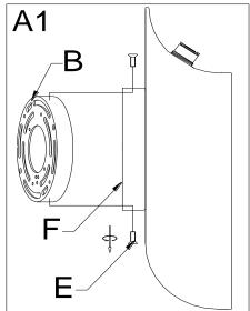
Separate the Mounting Plate (B) from the Canopy (F) by removing the Canopy Screws (E). Do not discard the Canopy Screws (E) as these will be used later.
