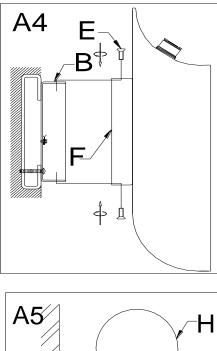
Position the Canopy (F) over the Mounting Plate (B), aligning the 2 holes on the Canopy (F) with the 2 holes on the Mounting Plate (B). Secure the Canopy (F) by tightening 2 Canopy Screws (E)
