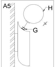
Attach the Glass Shade (H) onto the Socket (G) by rotating the Glass Shade (H) in a clockwise direction. Do not over tighten
