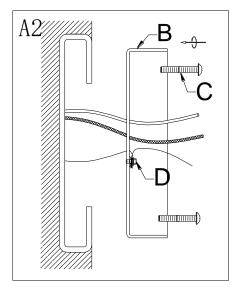
Insert the J-box wires through the center opening of Mounting Plate (B). Attach the Mounting Plate (B) onto the wall J-box.
