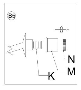
Unscrew the Socket Rings(N) and Spacers (M) from the Sockets (K) and Socket (Q) by rotating the Socket Rings (N) in a counter-clockwise direction.
