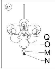
7. Attach the Glass Shade B (O) onto the Socket (Q) at the bottom of fixture. Place the Spacer (M) onto the Socket (Q), Secure Glass Shade B (O) and Spacer (M) by rotating the Socket Ring (N) in a clockwise direction until tight.
