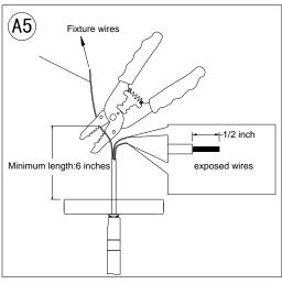
5. If needed, cut off the extra power cord length on the 3 wire cords so that they all are at least 6 inches (152.4 mm) long within the outlet junction box (J-box).
