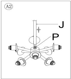
Insert the fixture 3 wire power cord through the 6 in. Tube (J), and attach bottom end of the 6 in. Tube (J) onto the Threaded Pipe (P) by turning clockwise until tight.
