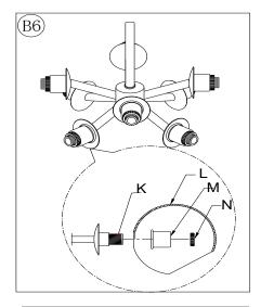
Attach the 8 Glass Shades A (L) onto the Sockets (K).
