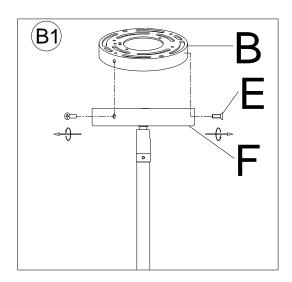
1. Separate the Mounting Plate (B) from the Canopy (F) by removing the 3 Canopy Screws (E). Do not discard the Canopy Screws (E) as these will be used later.
