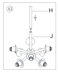
3. Take out three 12 in. Tubes (H) from poly bag. If you would like use only one 12 in. Tube (H), Then thread the 3 wire power cord through it, make sure the tube nipple joint end is downward. Attach the 12 in. Tube (H) onto the top of Short Tube (J) and rotate 12 in. Tube (H) clockwise until tight. Use the additional 12 in. Tubes (H) as needed, to adjust the fixture's suspension length using the similar procedure.
