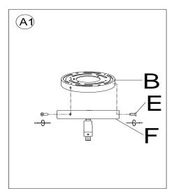
Separate the Mounting Plate (B) from the Canopy (F) by removing the 3 Canopy Screws (E). Do not discard the Canopy Screws (E) as these will be used later.
