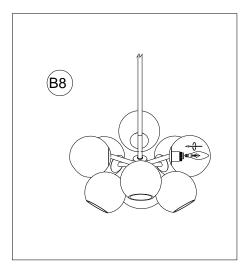
Insert the specified light bulbs into the Sockets (K) and Socket (Q). DO NOT EXCEED THE SPECIFIED WATTAGE.
