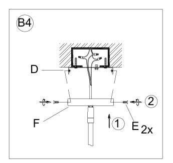
Raise Canopy (F) up over the Mounting Plate (D), align the holes on the Mounting Plate (D) with the holes on the side of the Canopy (F). Insert the 2 Canopy Screws (E) and tighten with a screwdriver.
