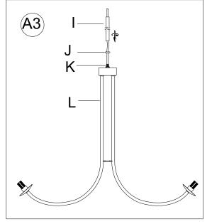
Insert the fixture 3 wire power cord through the Short Tube (J), and attach bottom end of the Short Tube (J) onto the Threaded Nipple (K) by turning clockwise until tight.
