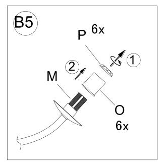
Remove Socket Rings (P) and Metal Spacers (O) by turning each Socket Ring (P) from each Socket (M) counter-clockwise, and set them aside.
