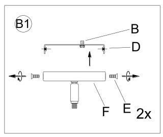
Separate the Mounting Plate (D) from the Canopy (F) by removing the 2 Canopy Screws (E). Do not discard the Canopy Screws (E) as these will be used later.
