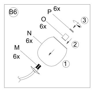
Position one Glass Shade (N) over one of the Sockets (M). While holding the Glass Shade (N) in place, place the Metal Spacer (O) onto the Socket (M) first and then turning the Socket Ring (P) clockwise onto the Socket (M) by hand until tight. Do not over tighten. Assemble each of remaining Glass Shades(N) onto each of Sockets (M) using the same procedure as above.
