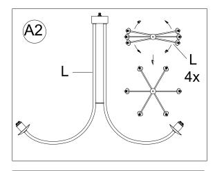
Carefully rotate each metal arms into their final position so they are equally spaced as shown in diagram.
