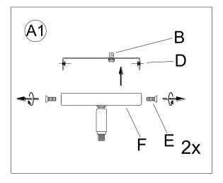
Separate the Mounting Plate (D) from the Canopy (F) by removing the 2 Canopy Screws (E). Do not discard the Canopy Screws (E) as these will be used later.
