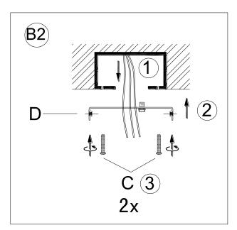
Gently pull existing wire down from the ceiling junction box and allow wires to hang. Attach Mounting Plate (D) to the ceiling outlet box. Tighten 2 Mounting Screws (C) with a screwdriver.
