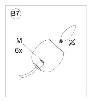
Insert the specified light bulbs into the Sockets (M). DO NOT EXCEED THE SPECIFIED WATTAGE.
