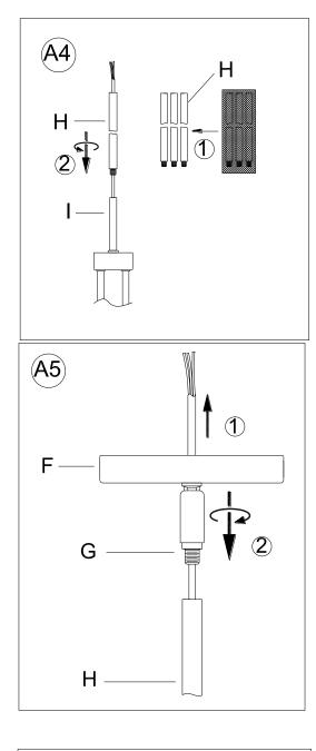
A6 Fixture wires 4. If you would like to use only one Long Tube (H), then thread the 3 wire power cord through the Long Tube (H), making sure the tube nipple joint end is downward. Attach the bottom end of Long Tube (H) onto the top end of Short Tube (I) and rotate clockwise until tight. Use the additional Long Tube (H) as needed to adjust the fixture's suspension length by following the similar procedure as outlined in step 1 of this illustration.
