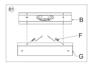
Separate the Mounting Plate (B) from the Canopy (G) by removing the 4 Canopy Screws (F). Do not discard the Canopy Screws (F) as these will be used later.
