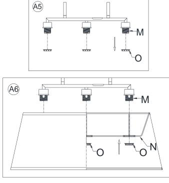
A7 /2inch exposed wires Winimum long /2inch 5. Unscrew the Socket Rings (O) from the Sockets (M).
