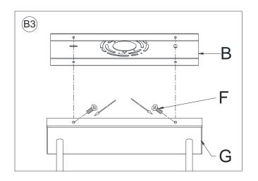
With the help of another person to hold the weight of the Chandelier, Raise the Canopy (G) up over the Mounting Plate (B), aligning the 4 holes from the Mounting Plate (B) with the 4 holes on sides of the Canopy (G). Insert the 4 Canopy Screws (F) and tighten each screw with a screwdriver until secure.
