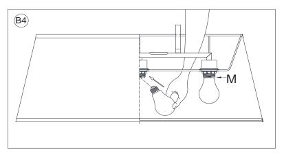
Insert the specified light bulbs (Not included) into the Sockets (M). DO NOT EXCEED THE SPECIFIED WATTAGE.
