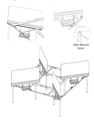
Step 10: Assemble Worksurfaces. Align Wedge Block under the Worksurface to hang over the back Frame rail. Push the Locking Handles in until handles are parallel with rail. Repeat 4 times.
