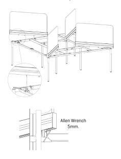
**Step 8: Assemble Wirebaskets.** Assemble 2 Hanger Column with the Wirebasket and Hanger Cap using enclosed M5 BHCS.
