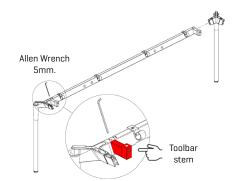
**Step 4:** Attach 1 outside leg assembly to the center H Frame using enclosed M8 SHCS.
