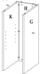
3. Carefully lift pre-assembled panels (K,G,H) onto bottom panel (E) by aligning cam bolts (A) with pre-drilled holes in panel (K), (G) and (H). Put cam houses (B) into pre-drilled holes in panel (K), (G), and (H) as shown. Tighten all cam houses (B) with allen key (D).
