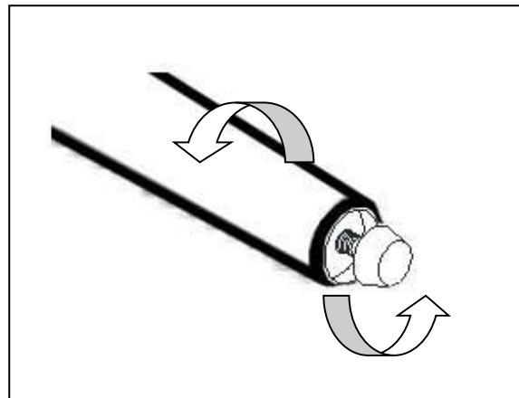
1. If the floor is uneven, adjust the recessed levelers found on the bottom of the furniture.
