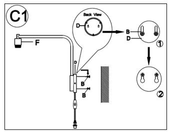
Preferably with the help of another person, lift the lighting fixture against the wall so the two mounting keyholes on the Mounting Plate (C) align with and engage the protruding screw heads (B). Gently lower the lighting fixture so that the screws support its full weight. Make sure that each screw (B) is completely engaged with its keyhole before releasing the fixture.
