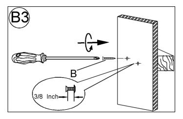
3. Use the Phillips screwdriver to secure the Wall Screws (B) into each drilled hole. Rotate the Wall Screw (B) clockwise until the screw head is about 3/8 inches from the wall.
