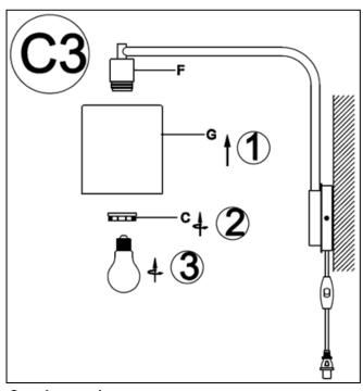
Place the Lamp Shade (G) onto the Socket (F). Secure the Lamp Shade (G) by turning the Socket Ring (C) onto the Socket (J) in a clockwise direction until tight. Insert the specified light bulb into the Socket (F). DO NOT EXCEED THE SPECIFIED WATTAGE.
