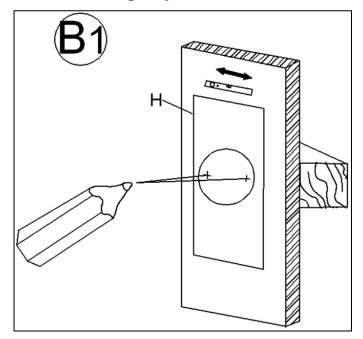
Place the Paper Template (H) against the wall at the desired hanging location. Mark the mounting location of the 2 holes of Paper Template (H) onto the wall using a pencil. Use a carpenter's level to ensure a level installation. MAKE SURE THAT A POWER OUTLET IS REACHABLE BY THE CORD without straining the cord.
