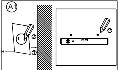
1. Place the Paper Template (H) against the wall at the desired hanging location. Mark the mounting location of the 2 holes of Paper Template (H) onto the wall using a pencil. Use a carpenter's level to ensure a level installation. MAKE SURE THAT A POWER OUTLET IS REACHABLE BY THE CORD without straining the cord.
