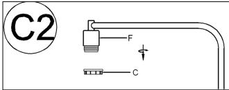
2. Unscrew the Socket Ring (C) from the Socket (F).
