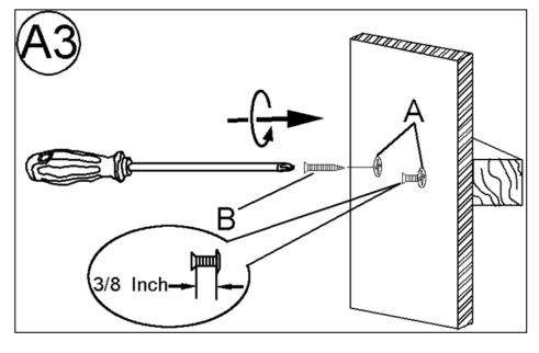
3. Use the Phillips screwdriver to secure the Wall Screw (B) into each installed Wall Anchor (A). Rotate the Wall Screw (B) clockwise until the screw head is about 3/8 inches from the wall.
